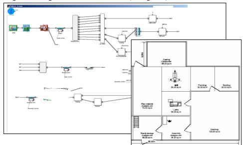
Figure 5. A snapshot of the DES-model for manufacturing of Attana 100's analysis units, and the corresponding layout of the workshop
