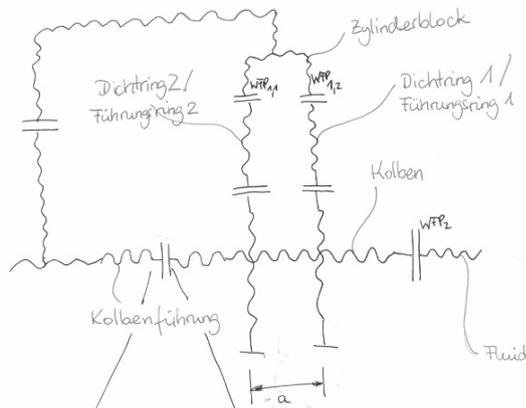
**Figure 5. Sketch of the C&CM structure of the product**
