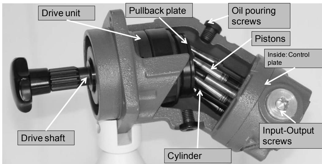
**Figure 1. Pump used in the experiment**
