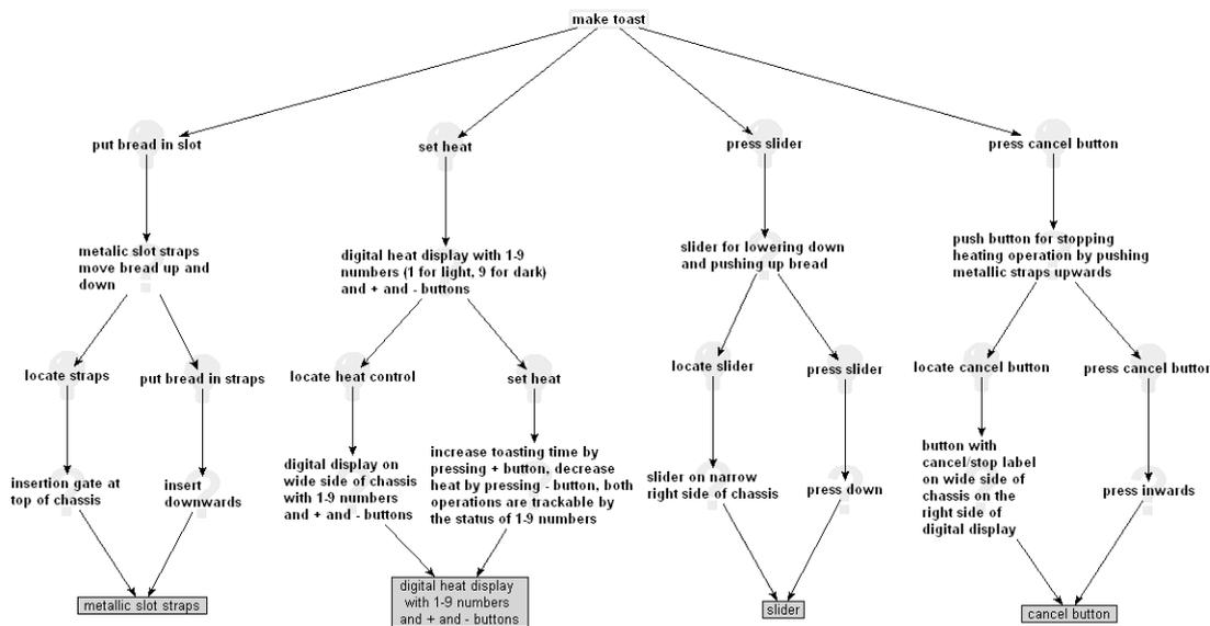
**Figure 2. Designer model of a simple toaster drawn using the new modelling approach in DRed**
