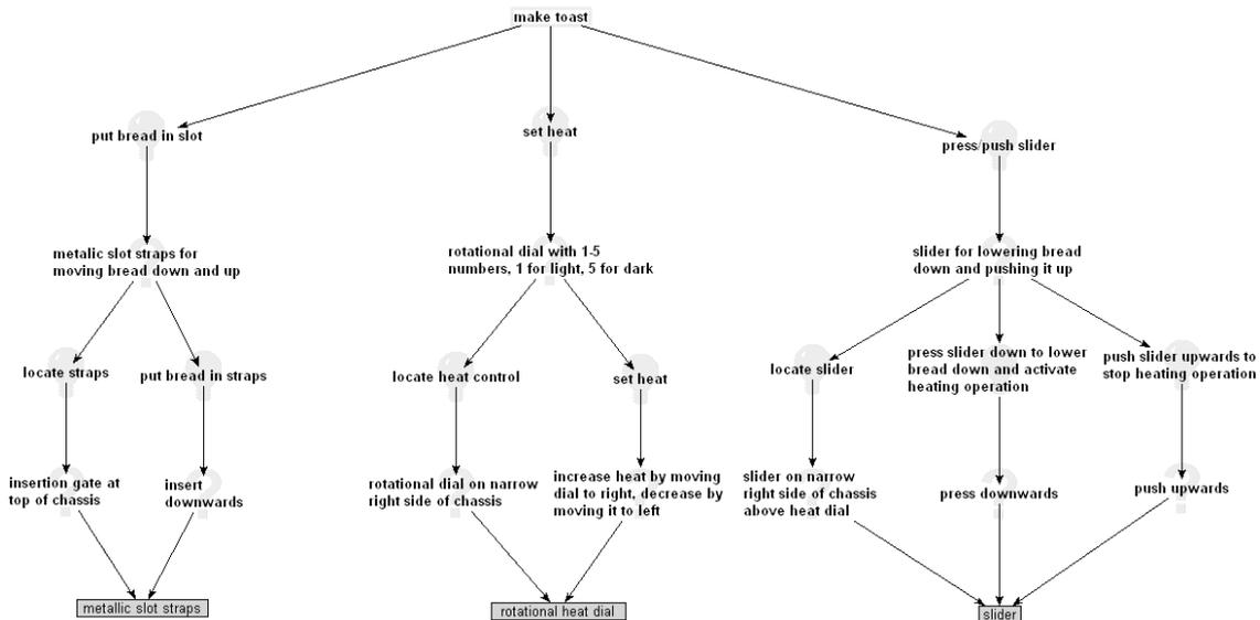
**Figure 3. User model of a simple toaster drawn using the new modelling approach in DRed**
