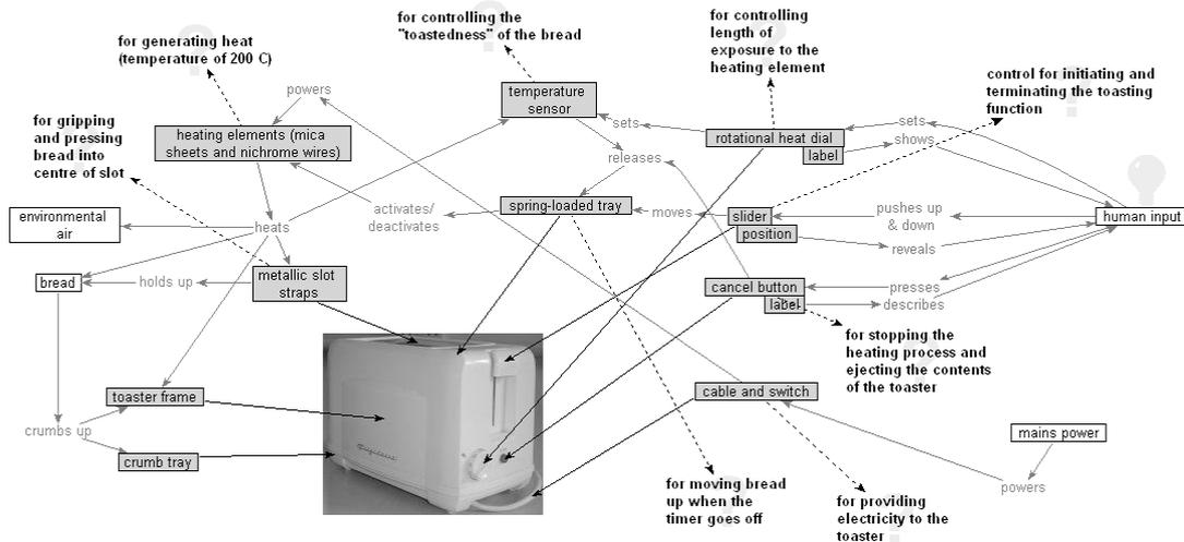
**Figure 1. Engineering model of a simple toaster drawn using the new approach in DRed**
