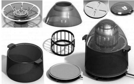
Figure 4. CAD modelling of redesigned pomegranate de-seeder by the authors
