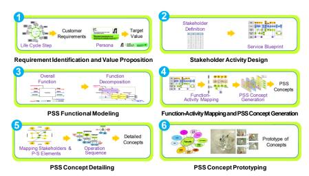
Figure 1 Product-Service Systems (PSS) design process (Kim et al., 2010)
