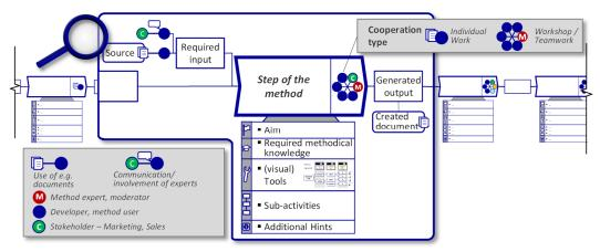
Figure 4. Method and Process Visualisation (MPV) cf. [Beckmann and Krause 2013]
