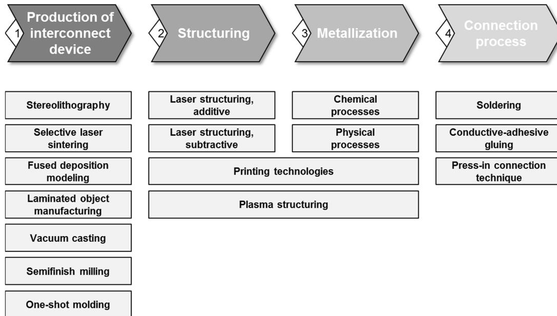
**Figure 4. Reference process for MID-Prototyping**
