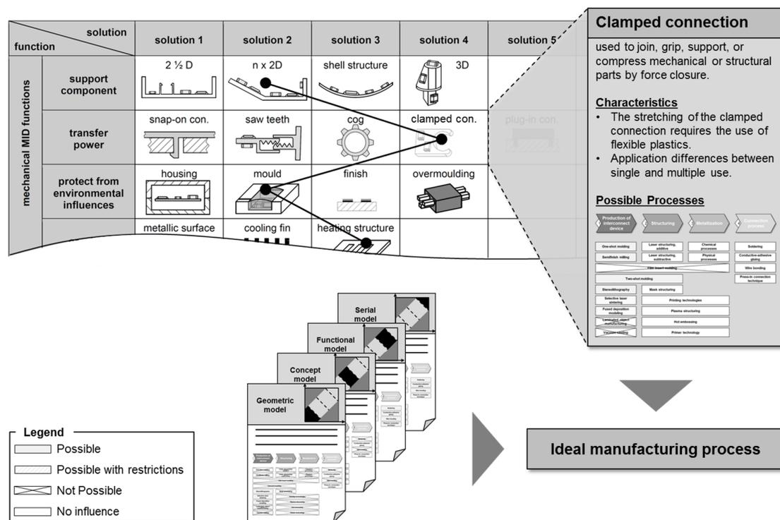
**Figure 8. Interaction of construction catalogue and general prototype classes**
