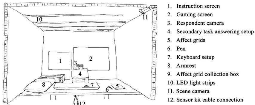
**Figure 4. Mockpit layout (for right-handed participant)**
