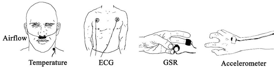
**Figure 3. Sensor placement (for right-handed participant)**
