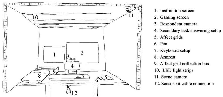
**Figure 1. Sketch of the Mockpit setup as it was used in the experiments (setup for right-handed participants). From Kittilsen et al. 2016 (in press)**
