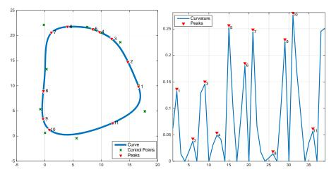
Figure 4. Left image: Cubic B-spline curve, its 8 control points shown as crosses. Right image: Function 1/r, maximum values highlighted with triangle markers
