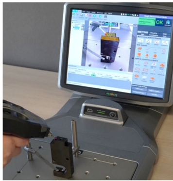
Figure 4. Geometrical measurement with a hand-held CMM with AR visualisation
