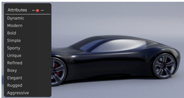
Figure 1. Example BlankAI tool offering control of form using semantic inputs for the attributes of AI-derived vehicle concept designs [3]
