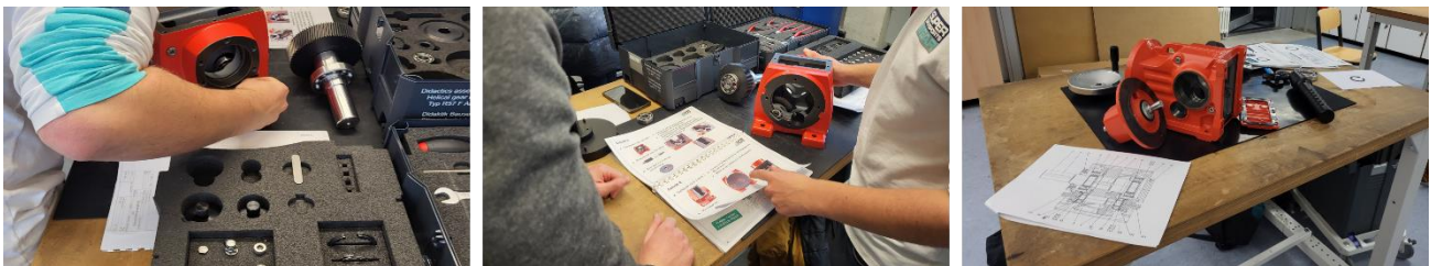
Picture 1. Assembly of the spur gearbox in the physical workshop
